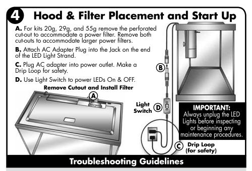
**NOTE:** The first time the LED light is turned on, it may take several seconds to light. If the light does not come on after one minute, please contact customer service at 1-800-526-0650. This delay should only occur the first time the light is used.
